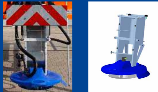
Stainless steel distribution system with mixing system
