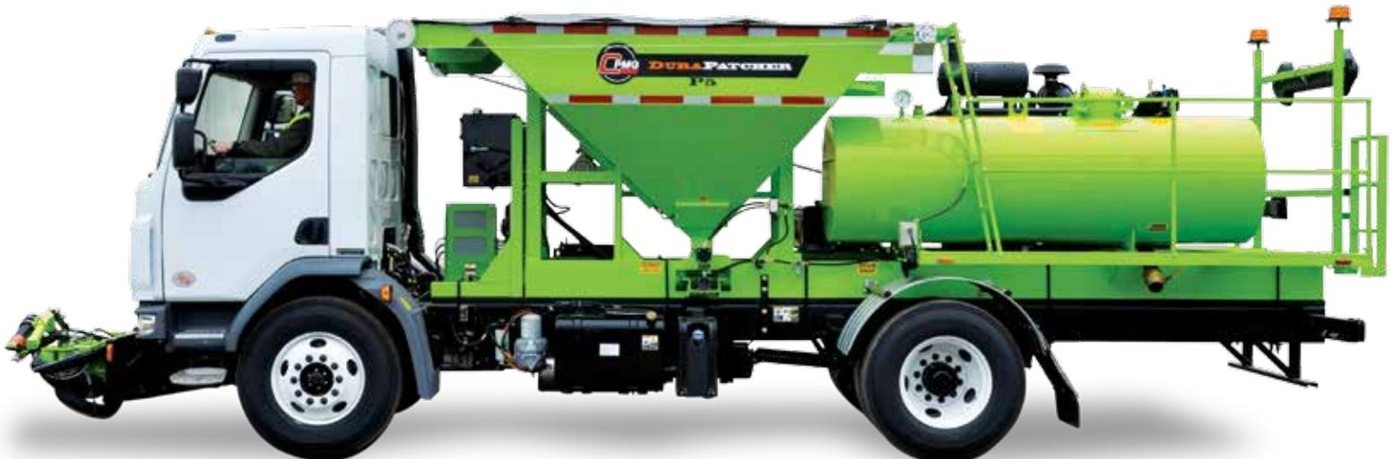
The covered five-yard aggregate hopper with vibrator feeds the venturi via dual air operated slide gates. The hopper is sized to allow 2 fills for every 1 fill of the emulsion tank.
