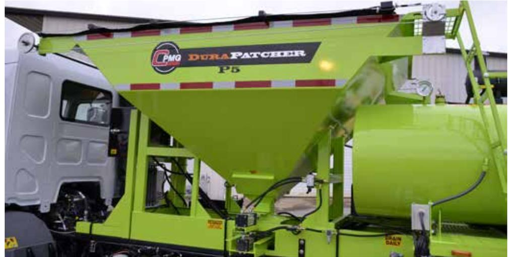
Dedicated diesel engine operates at pre-set low rpm and frees the truck engine to propel the vehicle.
