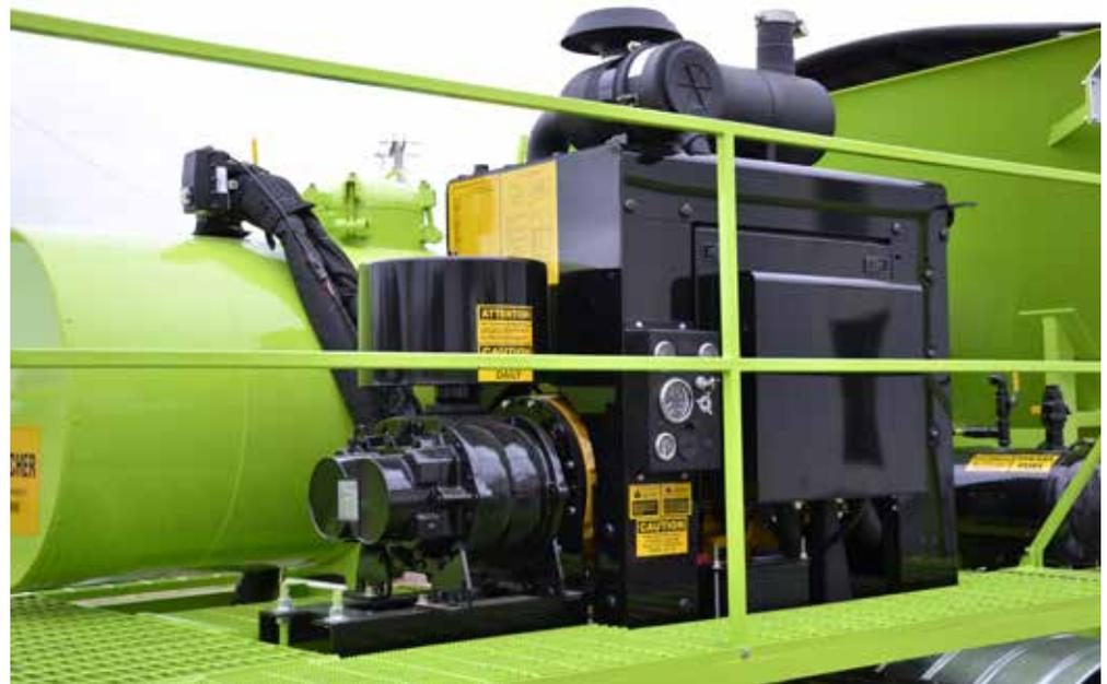
CAN-Bus technology is utilized throughout the system. This eliminates excessive wiring and is the industry standard for reliability, easy troubleshooting and repairs.
