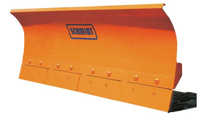
For narrow track vehicles when clearing small and medium amounts of snow.
