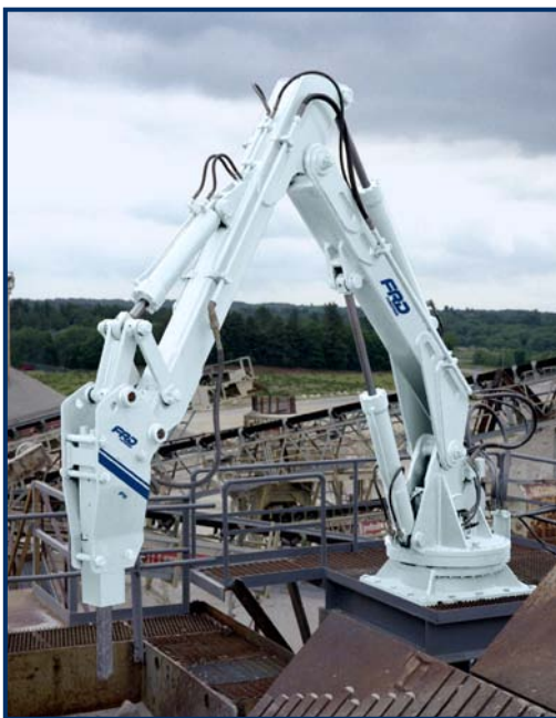
360° Rotational base for extended work envelope.
