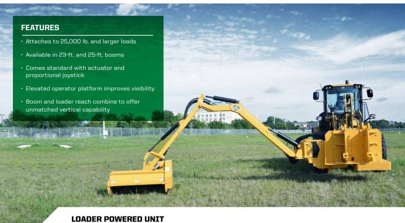
With no additional engine to maintain, this mower can be easily converted in the field to trim tree branches, cut brush or grass – and do it all from either the left or right hand side.
