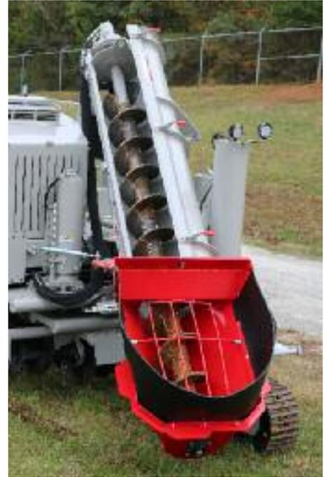
Auger Conveyor; lid opens for cleaning.
