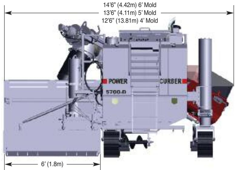
Machine with a 6' (1.8m) wide Sidewalk Mold.
