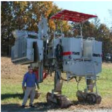
5700-D-MAX equipped with barrier mold lift.
