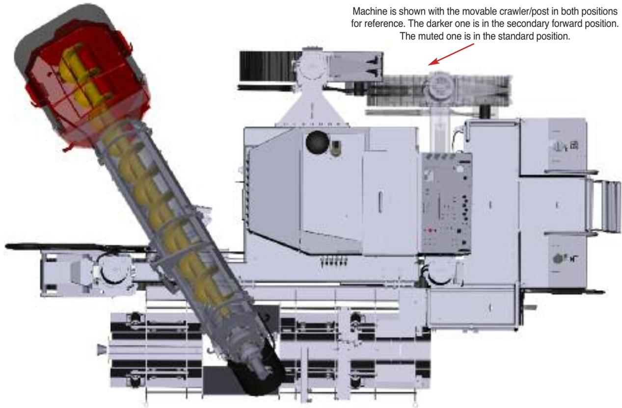
Machine is shown with the movable crawler/post in both positions for reference. The darker one is in the secondary forward position. The muted one is in the standard position.
