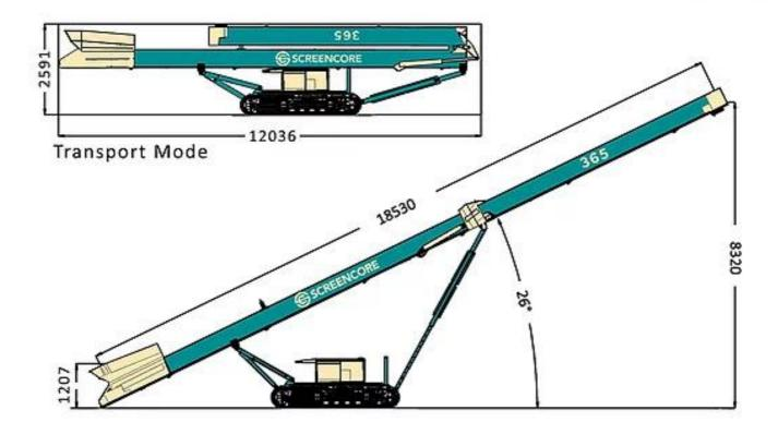
The Screencore 365 is a heavy-duty 65'(19812mm) x 3'(914mm) tracked stockpiler designed for convenient and efficient material movement and stockpiling.
