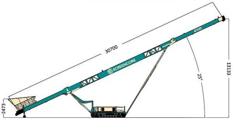
The Screencore 4100 is a 100' tracked stockpiler with 1200mm belt and a discharge height allowing for a conical stockpile of over 13m
