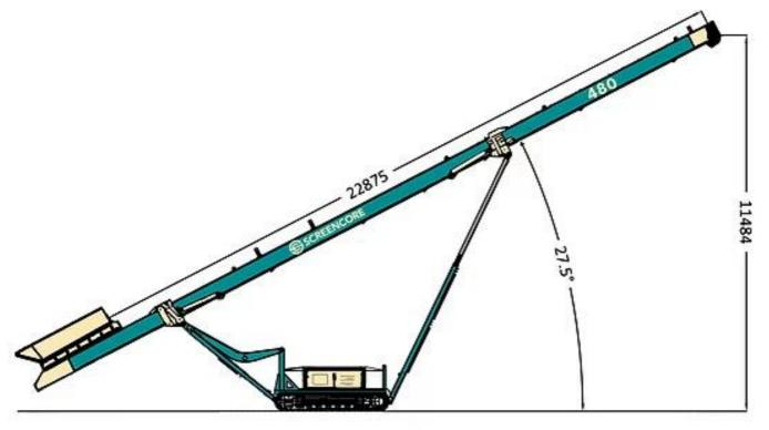
The Screencore 480 is an 80' tracked stacker with twin drive, 1200mm belt and extended feed hopper.
