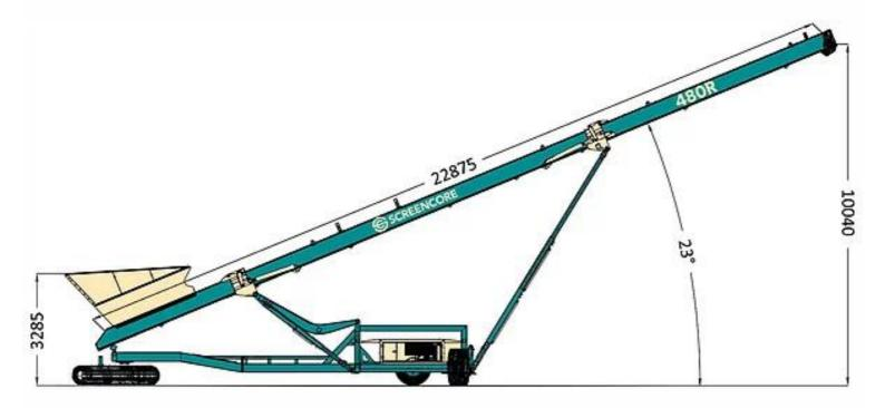
The Screencore 480R is an 80' radial tracked stacker with twin drive 1200mm belt for massive material movement and precise product placement.
