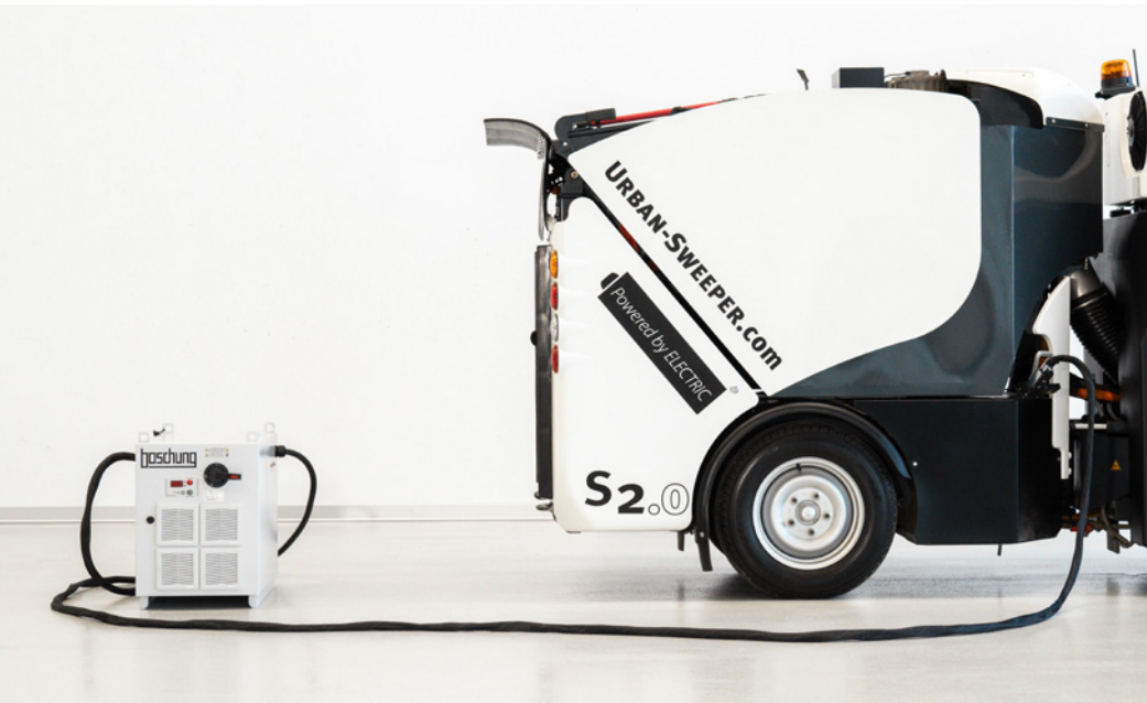
SuperCharger for a fast charging time of 100 minutes
